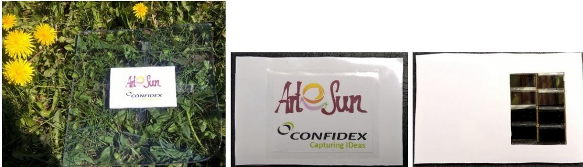
Figure 1: The RFID-OPV device is essentially a flexible label, ready to be attached on both opaque and transparent platforms. The credit card size OPV is powering the integrated sensor and boosting the communication between the reader and the tag.
