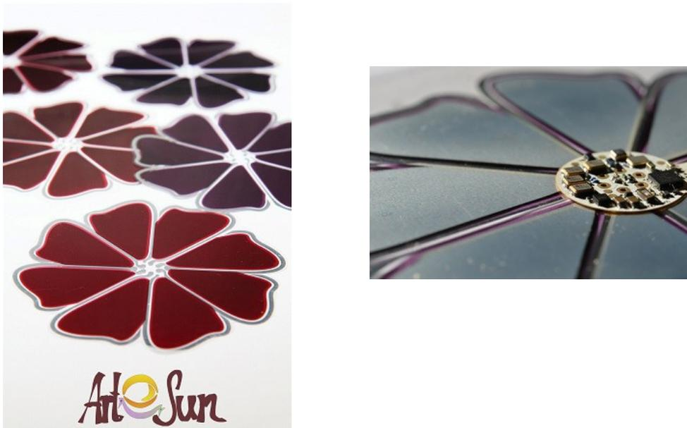
Figure 2: aesthetically pleasing flower-like organic solar module, realized by gravure printing to power the sensor device in a distributed wireless network node
